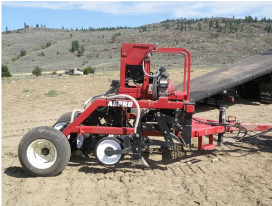
Figure 1: Ag-Pro drill used for no-till planting of winter Canola.
